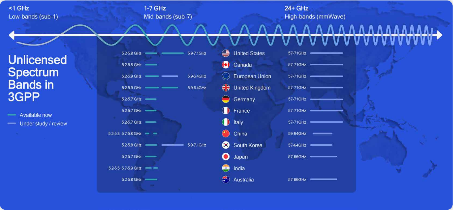
Figure 4.5 5G NR-U standardized in 5G NR Release 16. The first global cellular standard with both license-assisted and standalone use of unlicensed spectrum (Source: Qualcomm)
